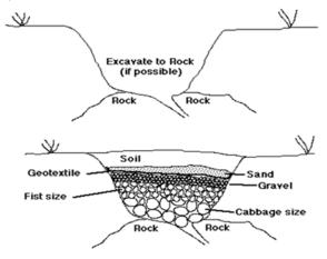
A sinkhole is best repaired by excavating to rock then building an aggregate filter in the hole, however, our area has little rock.
